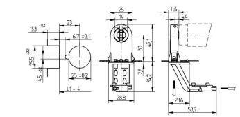
L1-4: Recommended dimension - The distance between the cutouts and the tolerance should be governed by the dimensions of the respective lamps and luminaires.
